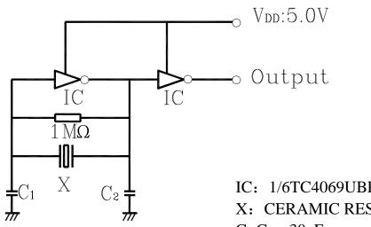
IC: 1/6TC4069UBP×2 X: CERAMIC RESONATOR C<sub>1</sub> C<sub>2</sub>: 30pF
